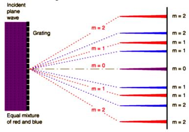
When a parallel beam of monochromatic light is directed normally (at right angles to it!) at a diffraction grating, light is transmitted by the grating in certain directions only.
