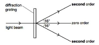
Fig. 2.2 does not show all of the emerging beams from the grating. The angle between the second-order emerging beam and the central zero-order beam is 16°.
